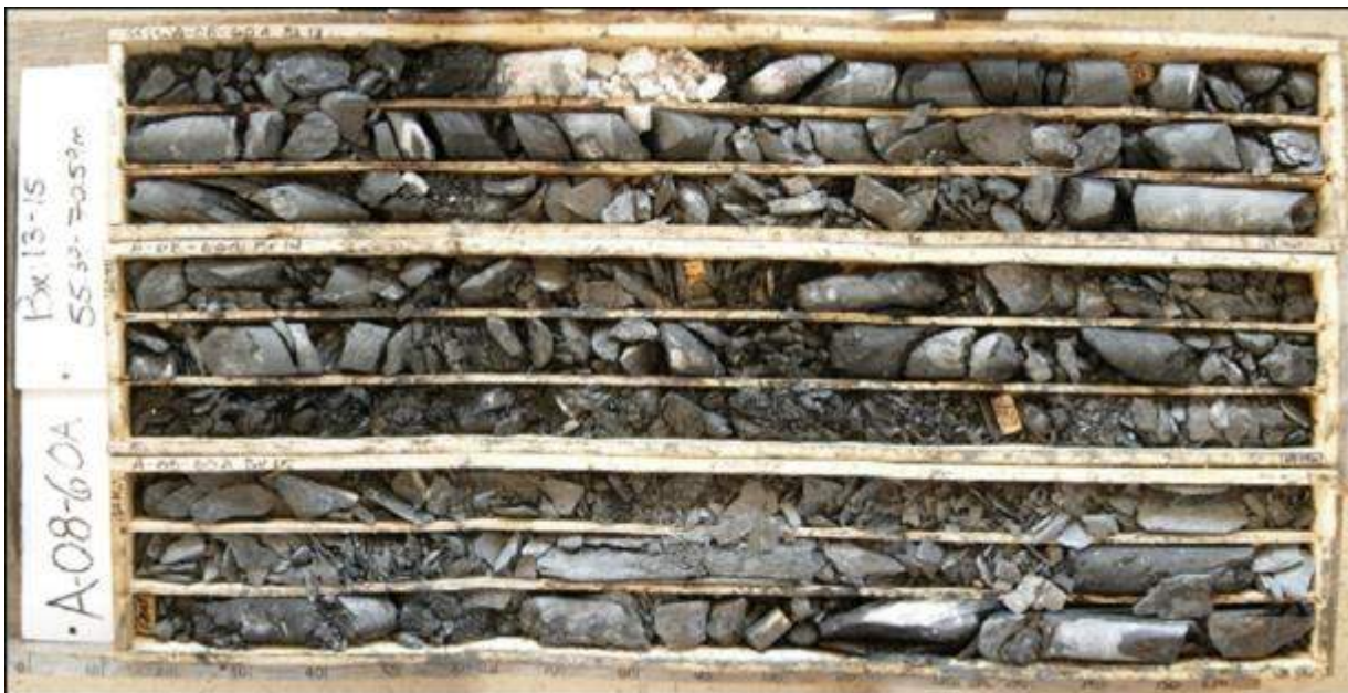
Figure 10-22: Bad Ground Associated with Brittle Faulting (A-08-60A)
