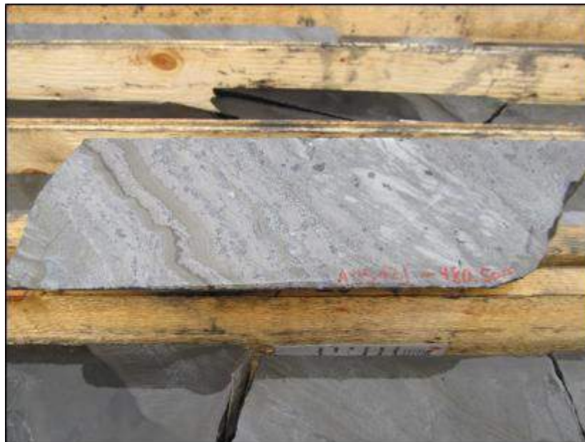
Figure 10-15: Mottled Textured High-Grade Mineralization in A-15-121 @ ~480.50 m
