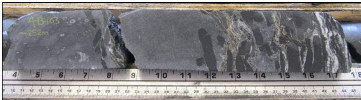
Figure 10-12: “Nick” Style Mineralization in Hole A-13-103 @ 252.37m
