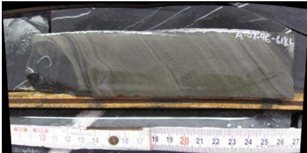
Figure 7-10: Sphalerite Banded Proximal Facies Mineralization in A-07-46 @ 618.60 m
