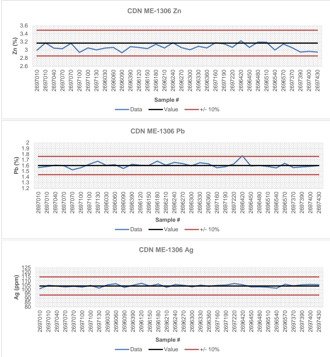
Figure 11-3: SRM Results from CDN ME-1306 for Zinc, Lead and Silver
