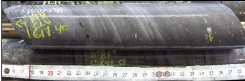
Figure 7-12: High-Grade Sphalerite Mineralization Interbedded with Barite in A-10-73B @ 617.40 m
